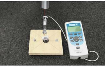
Testing of fixing element strength
